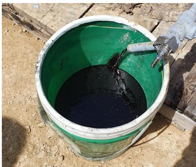
*Figure 3 - Sampling oil recovered at surface for lab analysis*
