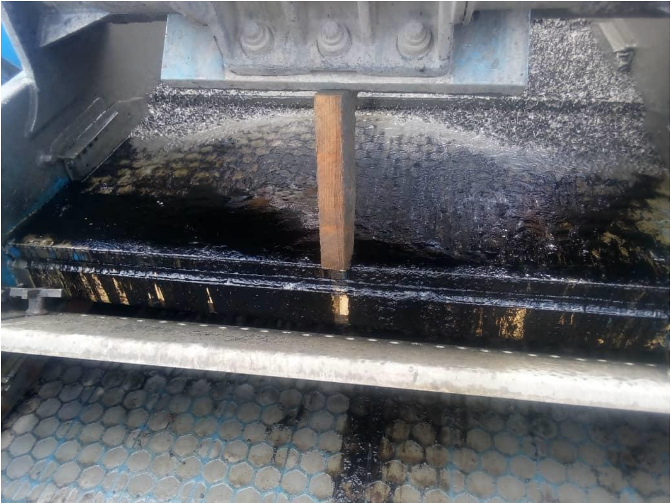
Figure 1 – Oil on shakers whilst drilling Zapato-1
