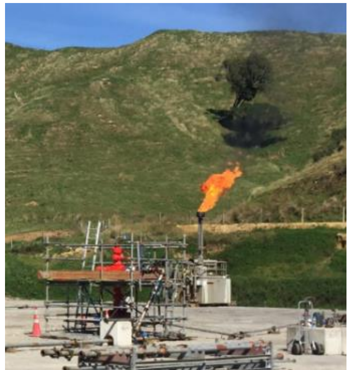
Figure 1: Oil associated gas being flared during the successful Pukatea-1 oil production test
