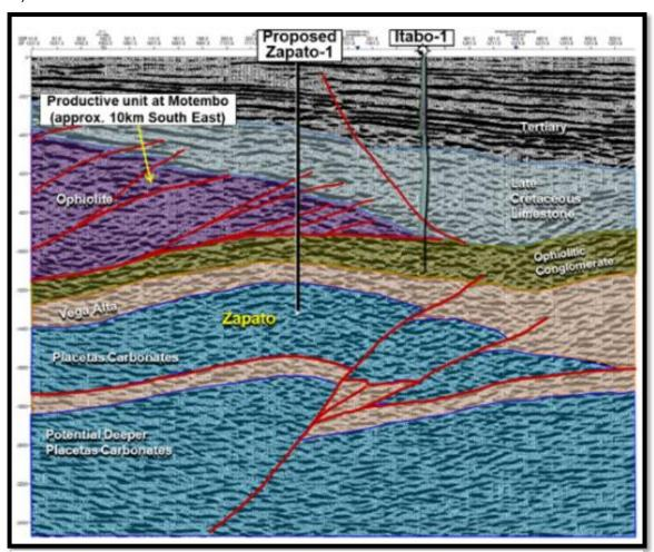
Figure 11 - Zapato prospect seismic profile and well path
