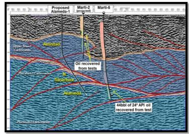
Figure 10 - Alameda-1 trajectory tests three objectives
