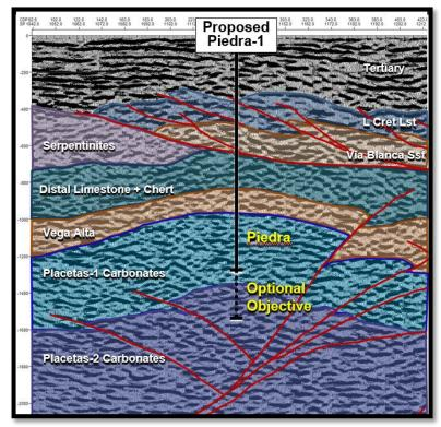
Figure 13 - Piedra prospect seismic profile and well path
