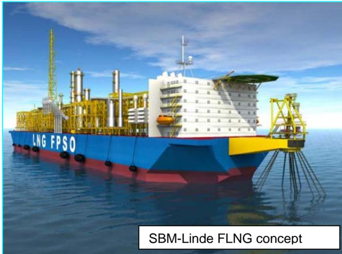
The floating LNG production concept is probably the quickest way to develop early production and cash flow for any new discovery. Commercial structures include leasing arrangements, with technical risk passed to the contractor. This could avoid major financing, technical and construction risk issues.
