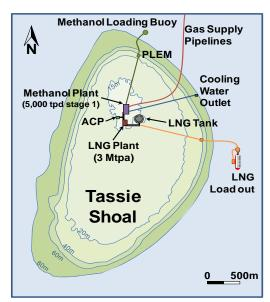
water cooling compared with air-cooling for a land-based plant. The balance of cost savings come from prefabricating and pre-commissioning the LNG plant and storage tank entirely in a low cost SE Asian construction environment and transporting the completed plant and tank directly to Tassie Shoal in single modules.
