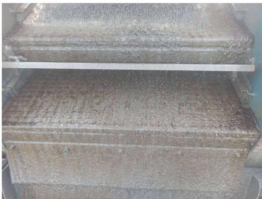
Oil on the shakers while drilling through Unit 1A.
