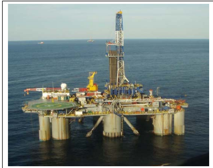
Songa Venus semi-submersible drilling rig
