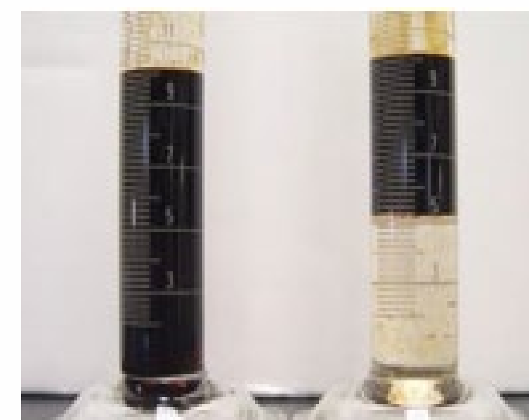
Melbana RDF was vigorously mixed with crude at reservoir temperature with separation in <30 mins.
