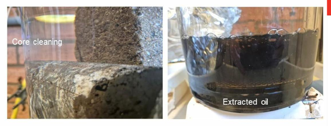
Oil extracted from Alameda 3 core that had no oil shows during drilling
