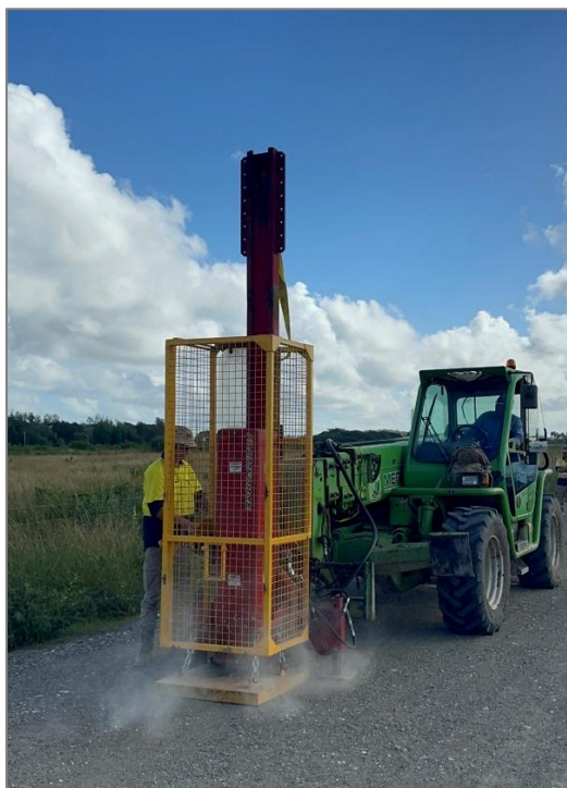
Figure 4 – “Thumper” weight-drop system in action
