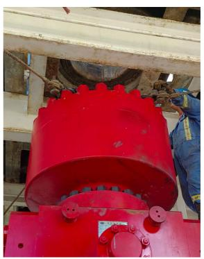
Figure 2 - BOP installed and tested
